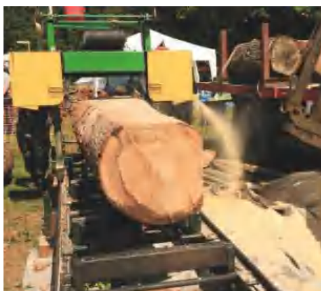
▲ Pic.6 The main trunk is sliced into boards on a horizontal bandsaw mill
